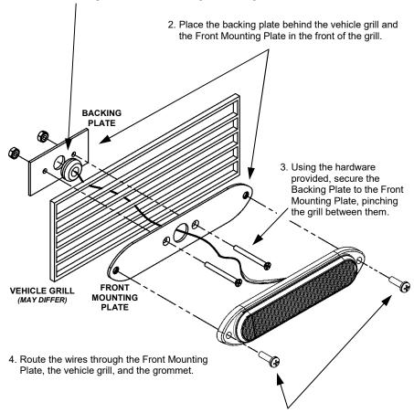
5. Use the screws shipped with this mounting bracket to mount the light to the threaded inserts in the Front Mounting Plate and make electrical connections according the instructions that came with your light.
